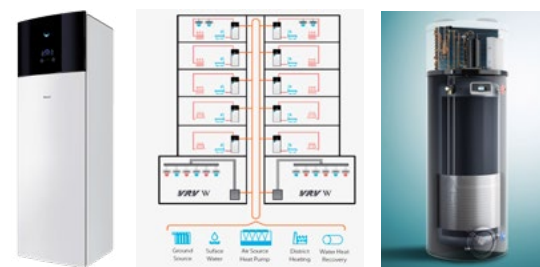
Fig 74: (L-R) Example heat pump (credit: Daikin); communal heat network schematic (credit: Daikin); DHW ASHP (credit: Vaillant)
