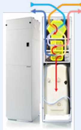
Fig 59: Example of MVHR+EAHP+DHW monoblock type unit (credit: Twinn Sustainability Innovation overlay on Nilan image)
